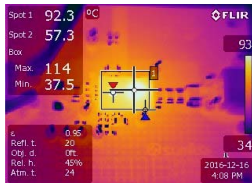
Fig. 15. Steady-state Thermal Image with 8A Load Current
