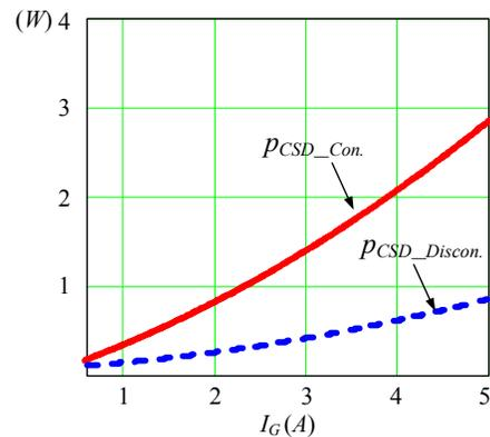
Fig. 5 Drive loss comparison between the continuous CSD and discontinuous CSD at 1MHz with different gate currents
