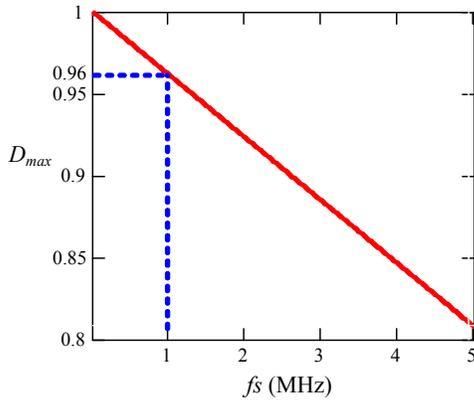
Fig. 11 The maximum duty cycle vs. the switching frequency
