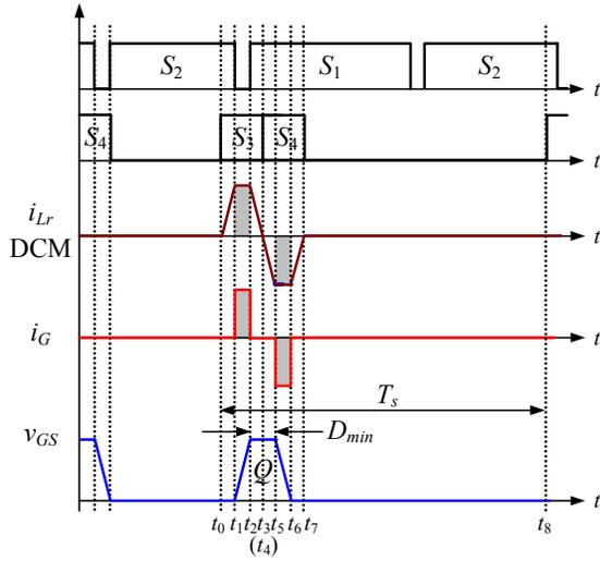
Fig. 8 Key waveforms with minimum duty cycle
