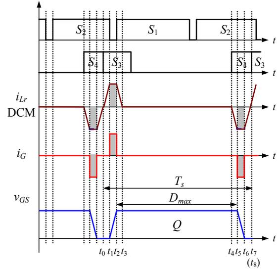
Fig. 10 Key waveforms with maximum duty cycle
