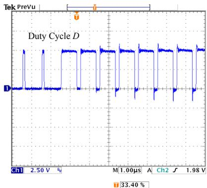
Fig. 14 Gate signals  $v_{GS\_Q1}$  from  $D=0.1$  to  $D=0.8$ : discontinuous
