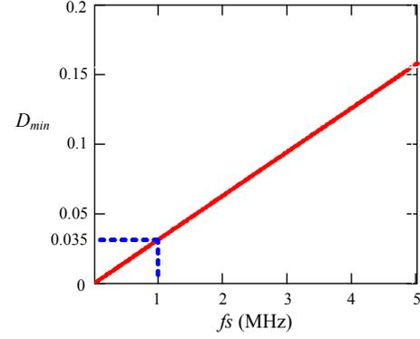
Fig. 9 The minimum duty cycle vs. the switching frequency
