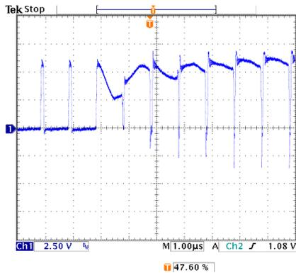
Fig. 13 Gate signals  $v_{GS\_Q1}$  from  $D=0.1$  to  $D=0.9$ : continuous
