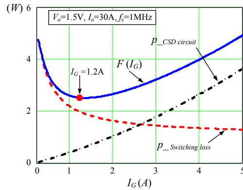
Fig. 7 Optimal function  $F(I_G)$  as function of current  $I_G$ : continuous
