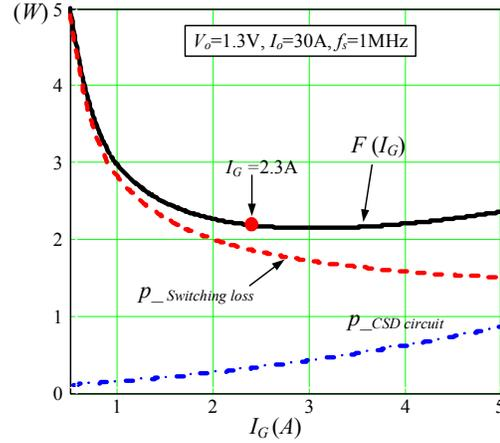
Fig. 6 Optimal function  $F(I_G)$  as function of current  $I_G$ : discontinuous
