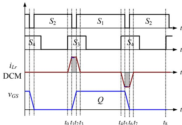
Fig. 4 Discontinuous key waveforms
