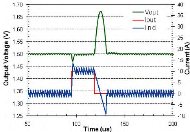
Fig. 13 Asymmetrical transient response to positive and negative load current step change
