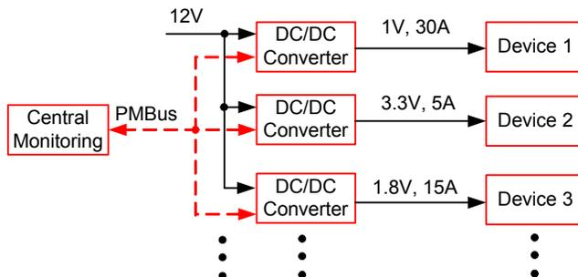
Fig. 2 PMBus Communication concept in multi-converter system
