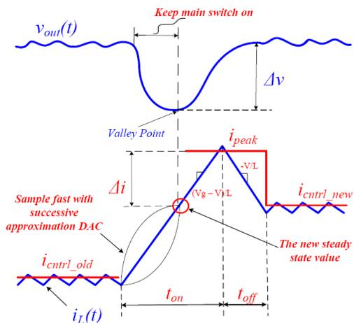
Fig. 12 The key waveforms of a single-phase power stage during a light-to-heavy load transient. Top: output voltage; Bottom: the inductor current.
