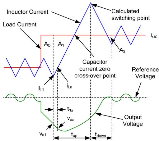
Fig. 9 CBC response under load step transient
