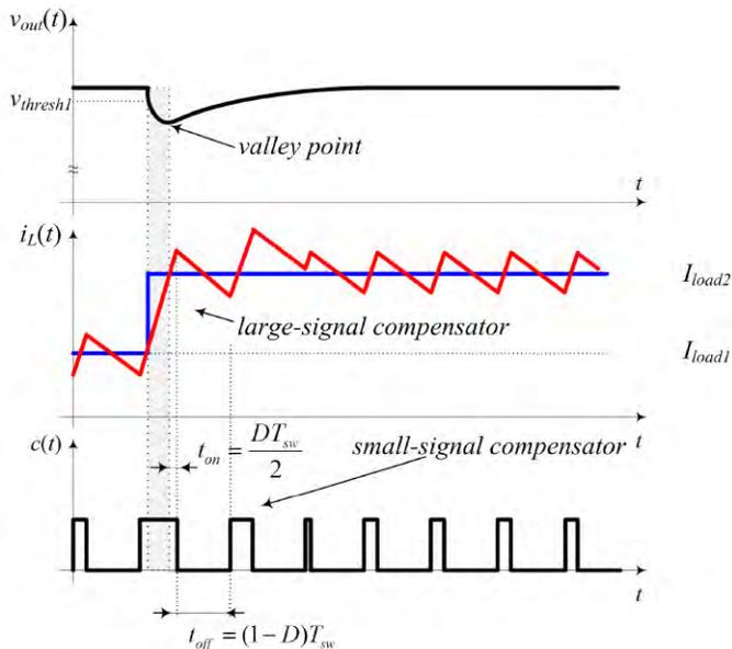
Fig. 11 Principle of operation of the “large-small” signal compensator during light-to-heavy with inserted control sequence
