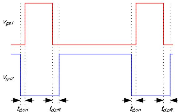
Fig. 3 Operation of a synchronous buck converter with dead time
