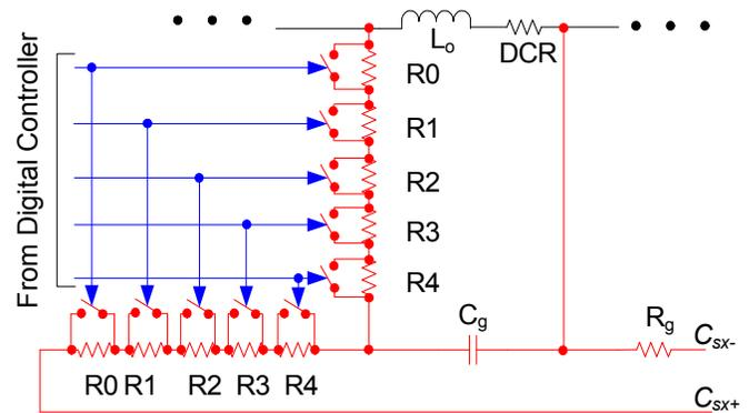
Fig. 5 Digital tuning of an analog  $RC$  inductor current sensor
