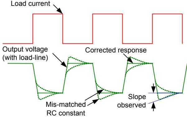
Fig. 6 Autotuning effect on a buck converter with load-line regulation
