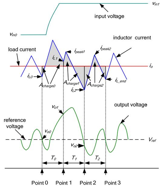
Fig. 10 Charge balance controller response to an input voltage transient
