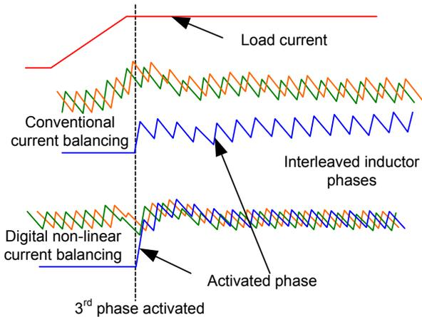
Fig. 4 Nonlinear digital phase balancing following phase activation.
