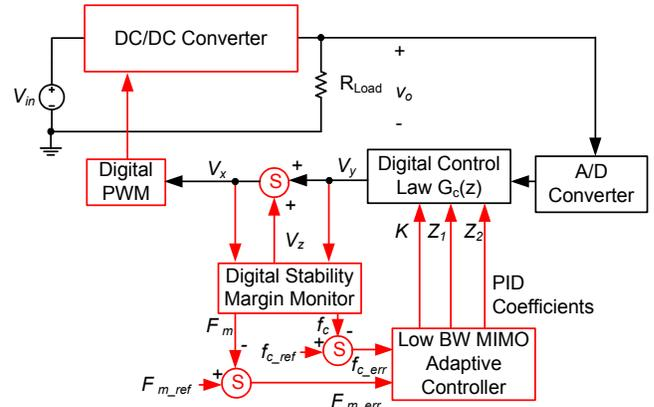
Fig. 8 Autotuning based on continuous phase margin measurement
