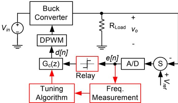
Fig. 7 Nonlinear relay to induce LCOs
