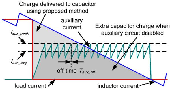
Fig. 14 Peak current mode, constant off-time operation of the proposed controller.
