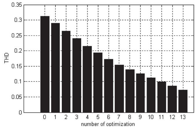
Fig. 3. THD of the input current after every optimization (full load = 1000 W).
