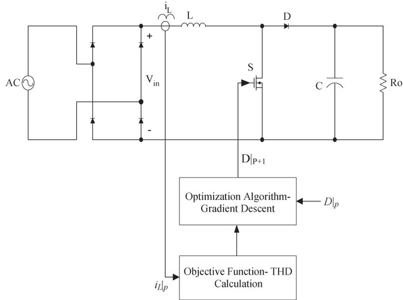
Fig. 1. Proposed new digital control PFC scheme.
