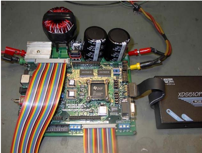
Fig. 6 Boost PFC circuit controlled by DSP evaluation board
