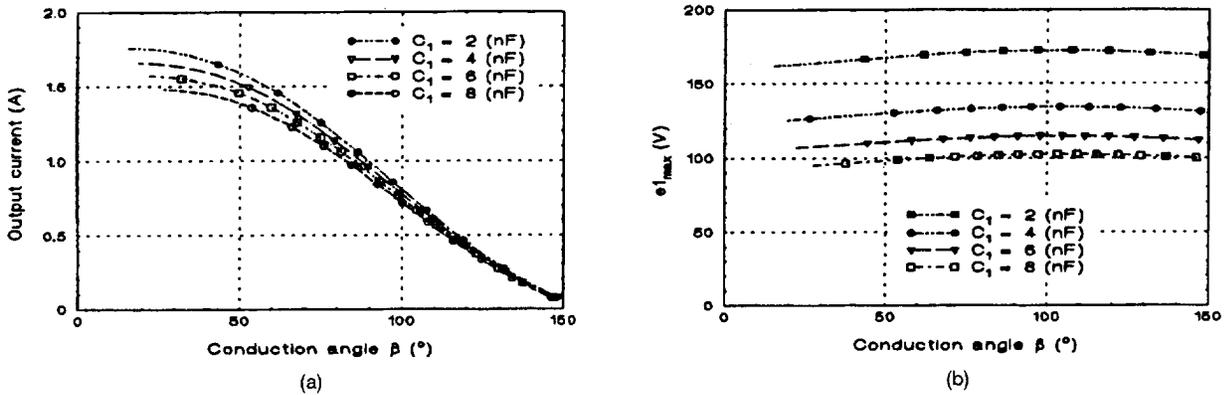
Fig. 10. Effect of parallel capacitor  $C_1$  on (a) output current and (b) voltage stress of  $S_1$  at  $V_s = 30$  V,  $V_0 = 30$  V,  $C_2 = 2.5$  nF,  $X = 10$   $\Omega$ ,  $f_r = 0.9$  MHz,  $f_s = 1$  MHz.
