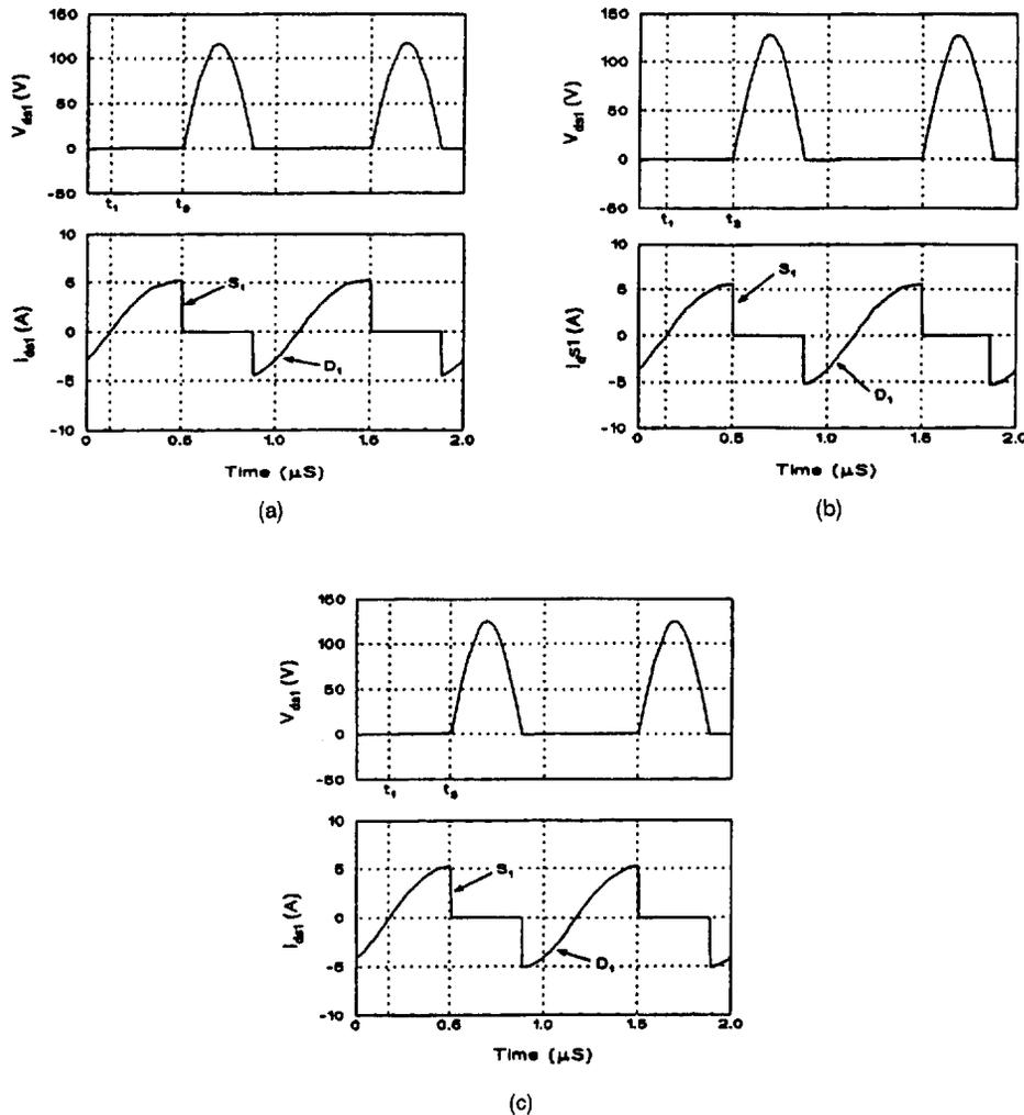
Fig. 13. Switching waveforms at  $S_1$  at different conduction angle  $\beta$ . (a)  $\beta = 0^\circ$ . (b)  $\beta = 90^\circ$ . (c)  $\beta = 144^\circ$ .
