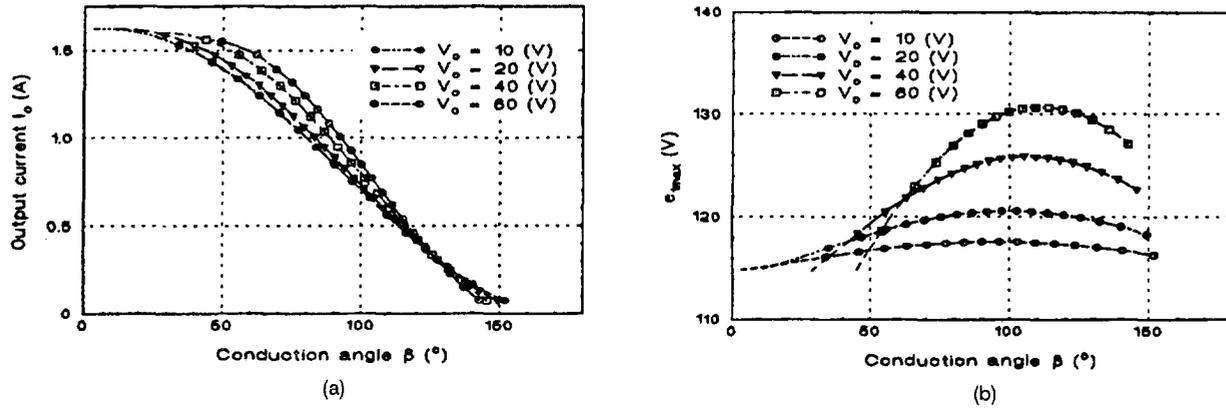
Fig. 8. Effect of output voltage on (a) load current  $I_0$  and (b) voltage stress of  $S_1$  at  $V_s = 30$  V,  $C_1 = 5$  nF,  $C_2 = 2.5$  nF,  $X = 10 \Omega$ ,  $f_r = 0.9$  MHz,  $f_s = 1$  MHz.
