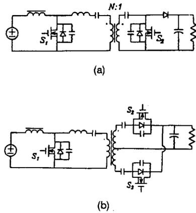
Fig. 12. Isolated version of class-E dc-to-dc converters with controlled current rectifier. (a) Half-wave. (b) Full-wave.
