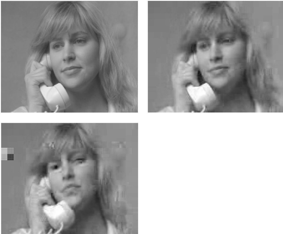
Fig. 7. Top-left: Original luminance frame 108 of Susie at 9.1 mbps/sec. Top-right: Susie at compressed 24 kbps in average shadowed fading channel at 12 dB SNR, 15 kbps, 145 ms delay channel. This top right image is visually indistinguishable from the case of an error-free channel. Bottom-left: worst-case channel distortion in 15 000 frames at 10 dB SNR, 15 kbps, 145 ms delay channel.
