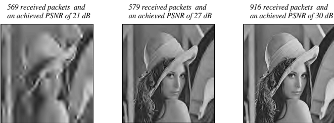
Fig. 3. The reconstructed Lenna images at an arbitrary class 2 receiver.
