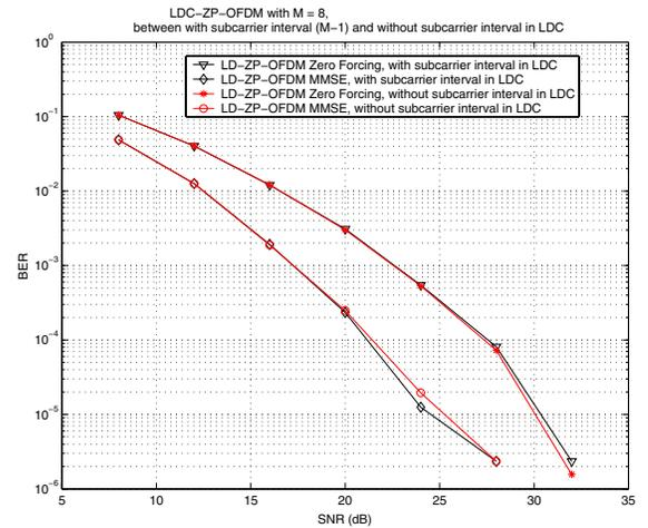
Fig. 5. For LDC-ZF OFDM, BER comparison between with subcarrier interval (M-1) and without subcarrier interval in LDC
