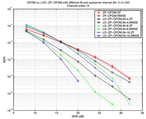
Fig. 4. BER Performance of OFDM vs LDC-ZP-OFDM with subcarrier interval
