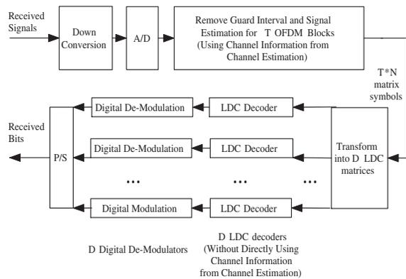
Fig. 3. Proposed LDC-OFDM receiver structure
