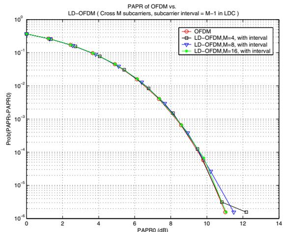
Fig. 6. PAPR performance of OFDM vs. LDC-OFDM
