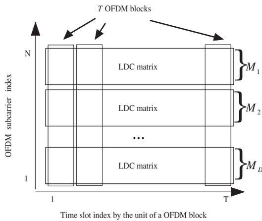
Fig. 2. LDC-OFDM blocks in the time-frequency plane
