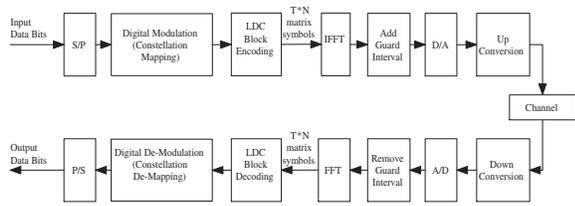
Fig. 1. Proposed LDC-OFDM system model
